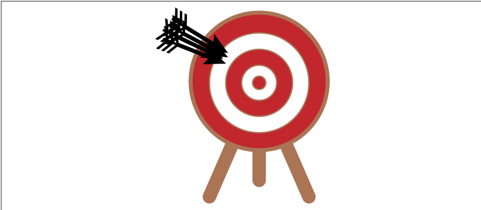
Figure 3-2. High-precision (but poor-accuracy) target shooting
