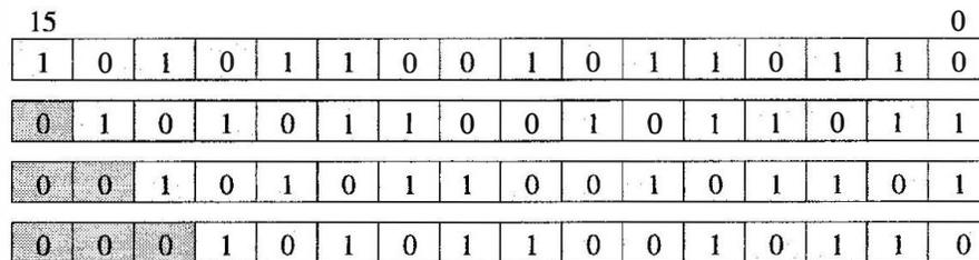
Figure 7.1: Shifting right 1 bit at a time (`shr`)
