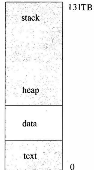
Figure 3.1: Process memory layout
